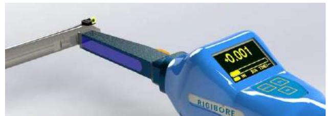
Note that there is approximately +/- 0.25 mm (on diameter) of fine adjustment available from the mid-adjustment position. The head must not be adjusted beyond this range.
