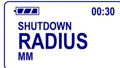
Use the *SEL* button to toggle between the 'RADIUS' and 'DIAMETER' display settings. To confirm the selection, press the *MENU* button once.
