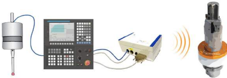
Fig.1- ActiveEdge tooling was integrated as part of a closed-loop process to improve accuracy and repeatability of bore sizes.
