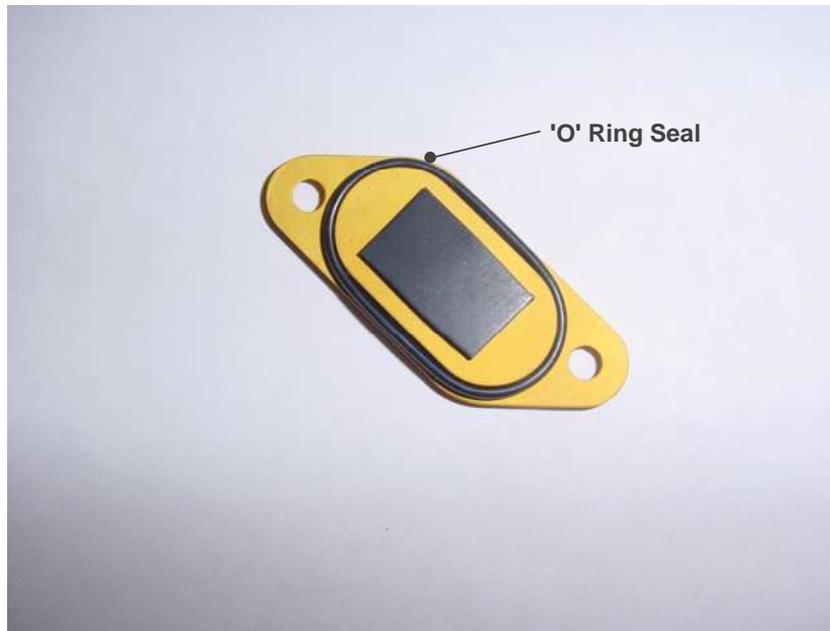
Ensure that the O-ring counterbore on the yoke cap is clean and free from debris.
